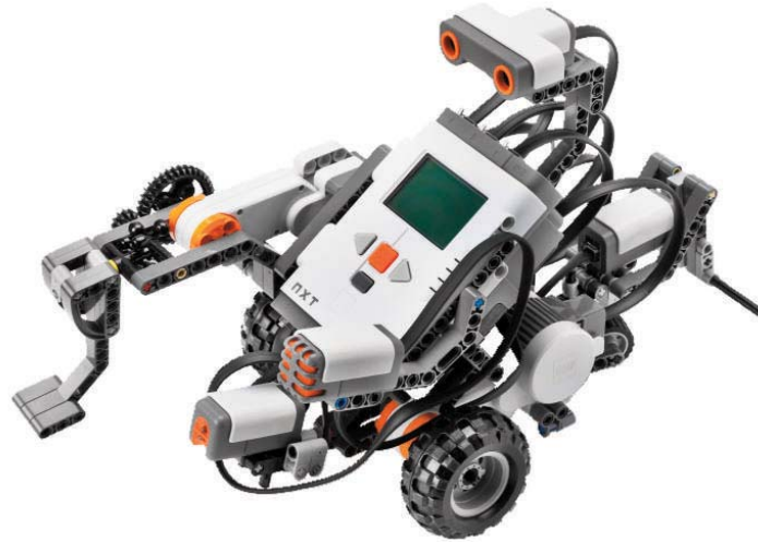
Figure 4 - A Lego NXT Roverbot with various sensors and motors.
